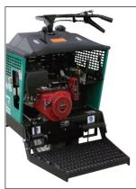
Operator's platform provides convenient access to all controls. Expanded metal floor plate provides secure footing and can be raised for storage or maneuvering in tight areas.
